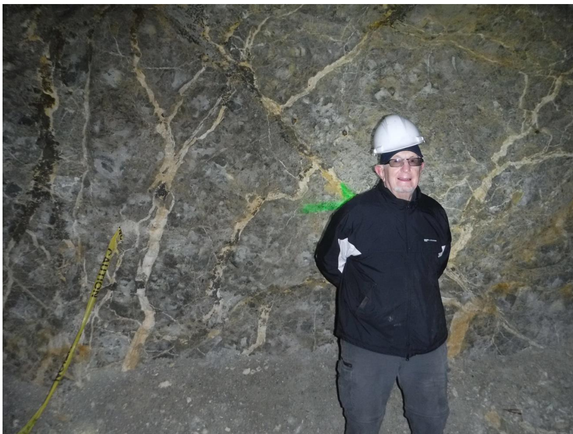
Stockwork Quartz Veins in Sandstone on the Lovitt Mine 1250 Level. Photo by J. Ebsich
